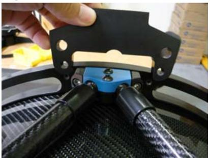
Attach the mounting bracket, with the radius at the bottom, to the CDK20 backplate using the two  $\frac{1}{4}$ - 20 x  $\frac{3}{4}$  button head cap screws (labeled 4 in figure 1) as shown in figure 2.
