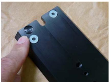
Place the dovetail on its back so that you notice the two spot faces (shallow counter bores) where the two small nylon washers are to be placed as seen in figure 4. Note: If you put a little grease on the washers then will stick in the spot face during assembly.
