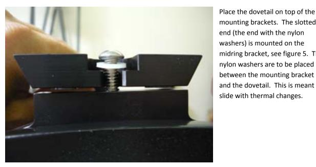
mounting brackets. The slotted end (the end with the nylon washers) is mounted on the midring bracket, see figure 5. The nylon washers are to be placed between the mounting bracket and the dovetail. This is meant to slide with thermal changes.
