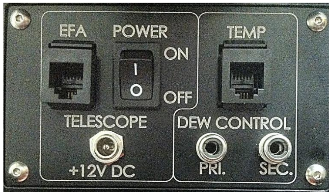
Fig 2 – Electronics panel on back plate of CDK12.5
