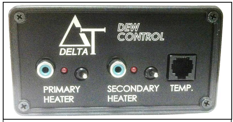
Fig 4 – Rear electronics panel on the Delta-T controller
