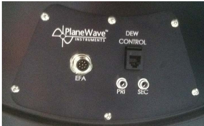
Fig 12 – Electronics panel on back plate of CDK17/20
