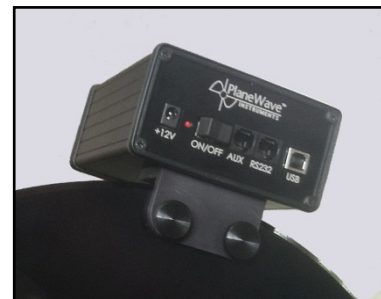
Fig 11– Delta-T Control box with mounting bracket and screws
