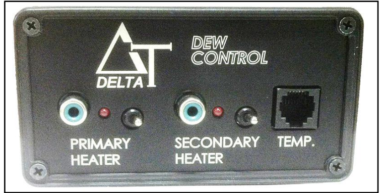
Fig 10 – Rear electronics panel on the Delta-T controller
