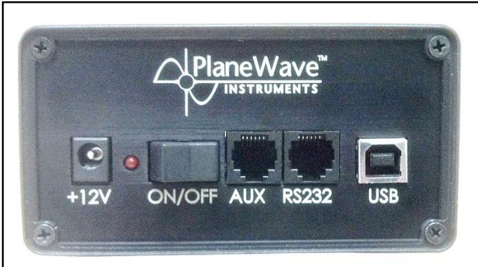
Fig 9 – Front electronics panel on the Delta-T controller
