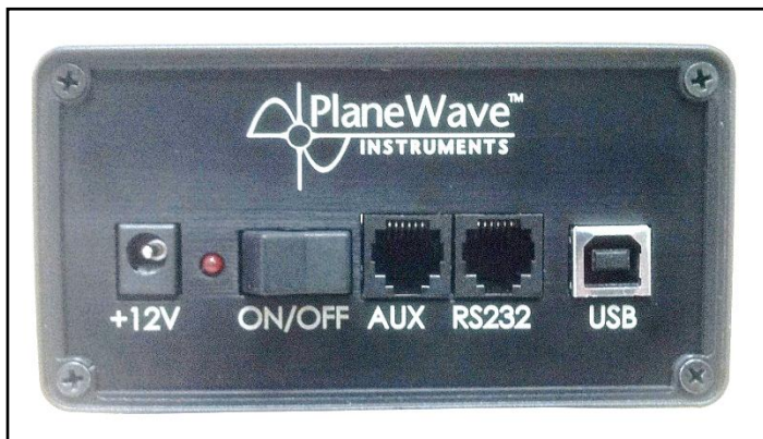
Fig 3 – Front electronics panel on the Delta-T controller
