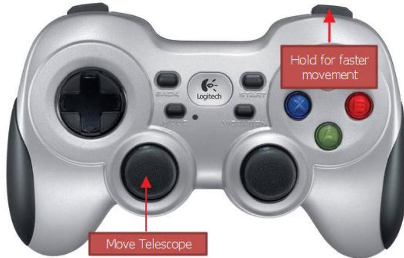
The maximum speed in Pan Mode is defined in the "Joystick Settings" window. By default the speed is 5 arcminutes per second, which is reasonable speed while doing visual observing of a standard target in the sky. If you would like to use the joystick to manually track a faster-moving object (such as a satellite or an airplane), you can increase this speed.
