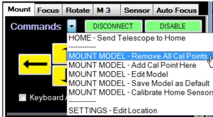
Next, make sure that sidereal tracking is turned ON and that the telescope is pointed at a clear part of the sky. Open the "Commands" menu and select "Add Cal Point Here".
