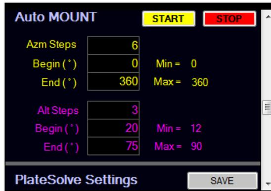
Click "START" to begin building a model using the specified parameters. The mount will slew to a series of locations, taking and PlateSolving an image at each location. For example, using the sample parameters shown above:
