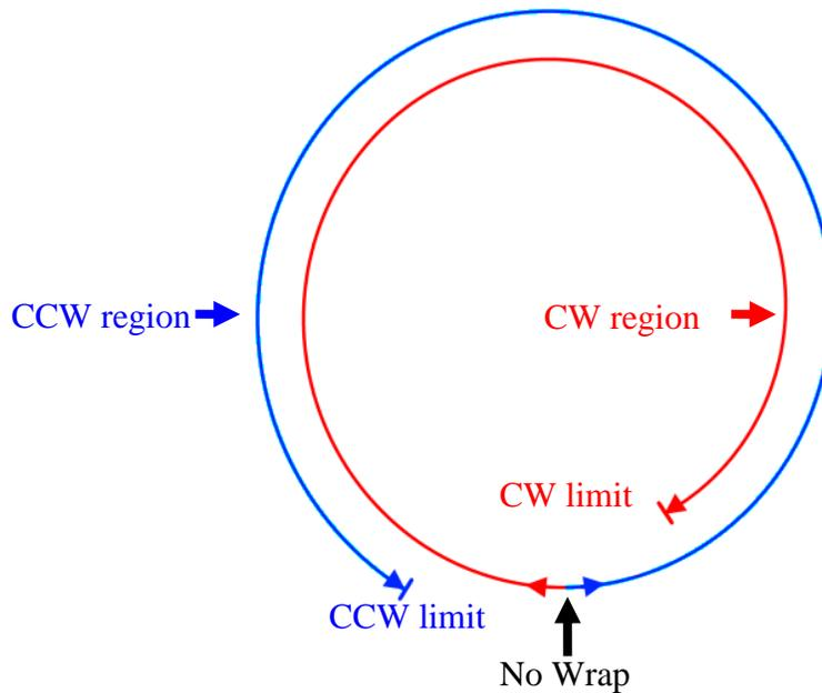
**Figure 6: Azimuth regions and range of motion, viewed from above looking down. In the Northern hemisphere, the "No Wrap" position would be oriented to the South. In the Southern hemisphere, "No Wrap" is oriented to the North.**
