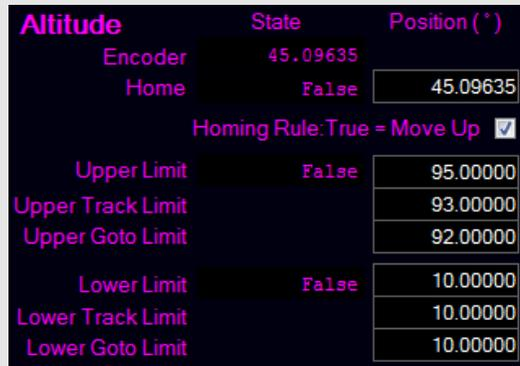
Once both axis home sensors have been calibrated, you should see that the "Home" setting under the Azimuth and Altitude sections of the "Mount Sensors" panel have been updated to the current position of the telescope.
