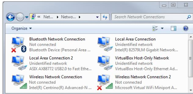
2. Identify which adapter is being used to connect to the CDK700. In general, it will be identified as one of the "Local Area Connection" options. The USB-to-Ethernet adapter is further identified in the screen below as "ASIX AX88772 US2.0 to Fast Ethernet".
