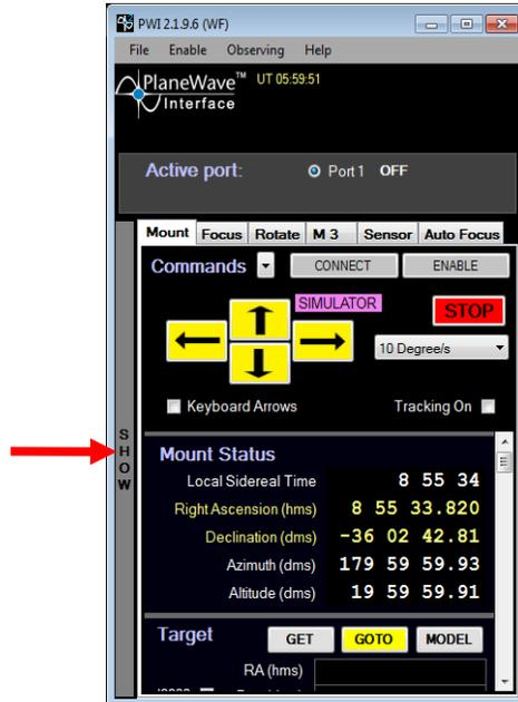
Figure 3: PWI window with Mount tab enabled
