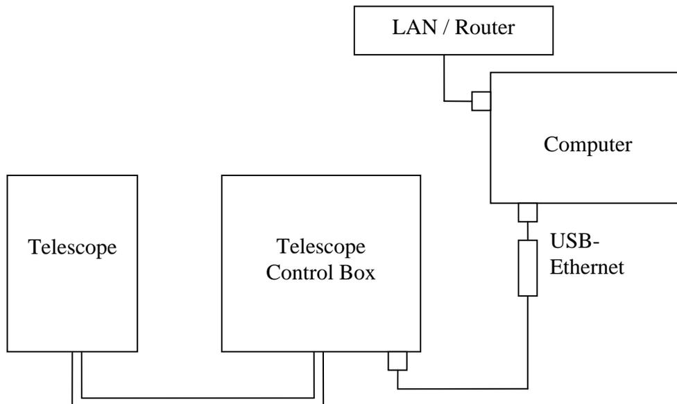
**Figure 2: Recommended connection layout**
