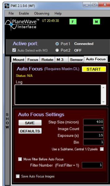
The Auto Focus routine will move the focuser to a series of evenly-spaced positions on either side of best focus and take images at those positions. It will then measure the diameters of all stars in each image and fit a model of star diameter versus focuser
