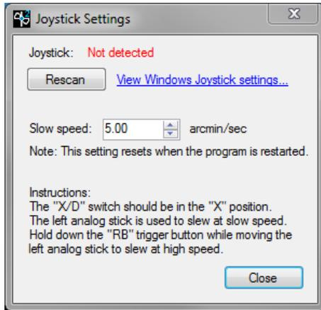
Click on the link to open the Windows Game Controller settings. Verify that the game controller is detected and correctly identified. Then click the "Rescan" button in PWI.
