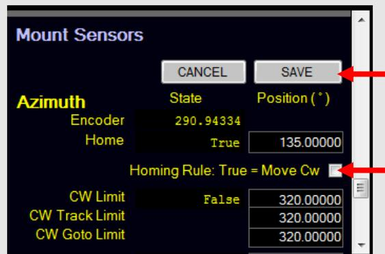
The homing sequence will approach the home sensor at 7 progressively slower speeds. The 7th and final approach is particularly slow in order to ensure high positioning accuracy. The whole process may take up to 3 minutes to complete. Once the Azimuth home sensor has been found, the OTA will rotate in Altitude to find the home position. Once again, the axis will approach the sensor at 7 progressively slower speeds before finishing.
