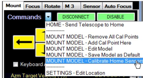
The mount will begin to rotate in azimuth towards the "No Wrap" position. Once this position is found, it will rotate towards the home sensor. The position of the sensor should be labeled with an arrow at the bottom of the mount.
