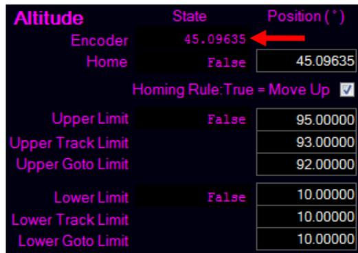
At this point it is safe to shut down the software and turn off the telescope. The next time you turn on the telescope and launch PWI, you will be able to quickly load the pointing model and calibrate the axis positions by finding the telescope home position.
