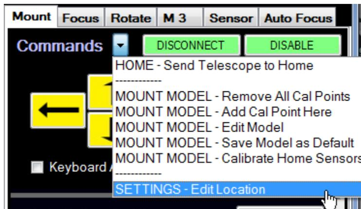
In the Mount Location window, enter the decimal longitude, latitude, time zone, and elevation of the telescope site.
