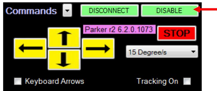
The first time you enable the mount axes after power-up, each axis will need to run through its automatic commutation procedure. This procedure takes approximately 30 seconds. During this time, you should see the Altitude and Azimuth coordinates change by small amounts in the "Mount Status" section:
