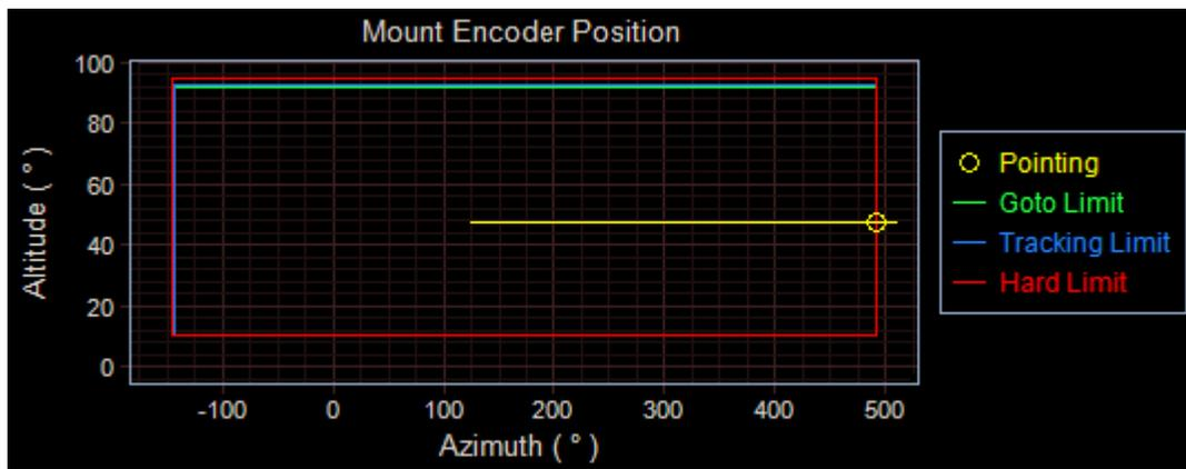
**Note:** In the Southern hemisphere (with No Wrap oriented to the North), the CW limit will be closer to 310 degrees.
