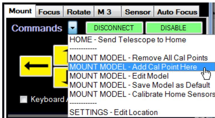
PWI will take an exposure from MaxIm DL and attempt to identify the image location using PlateSolve. If a solution is found, PWI will offset the axis encoder readouts to match the current telescope position as determined by PlateSolve. The status message at the top of the PWI window should report "Encoders have been set". Depending on how far off the initial mount position estimate was, you may see the pointing crosshairs and reported Altitude/Azimuth positions jump by several degrees.
