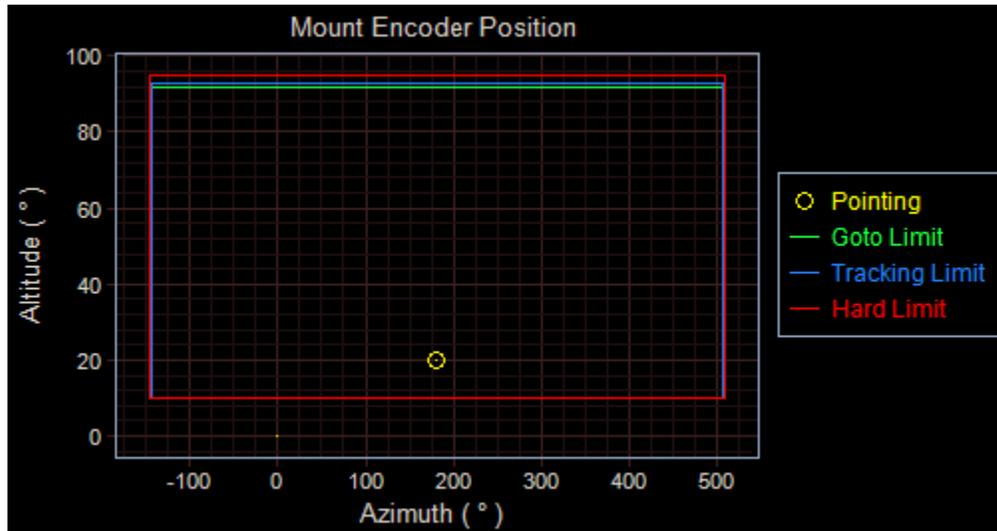
This graph also displays various limits for the position of the mount. On a Northern Hemisphere telescope the default limits should be approximately correct. On a Southern Hemisphere telescope they will be offset in Azimuth by 180 degrees. In either case, we will adjust the limits in the section below.
