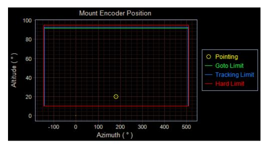
This graph also displays various limits for the position of the mount. On a Northern Hemisphere telescope the default limits should be approximately correct. On a Southern Hemisphere telescope they will be offset in Azimuth by 180 degrees. In either case, we will adjust the limits in the section below.
