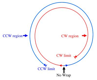
Figure 6: Azimuth regions and range of motion, viewed from above looking down. In the Northern hemisphere, the "No Wrap" position would be oriented to the South. In the Southern hemisphere, "No Wrap" is oriented to the North.
