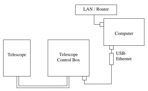
Figure 2: Recommended connection layout
