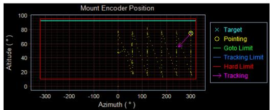
Figure 7: Mount position trace partway into an Auto Mount Model
