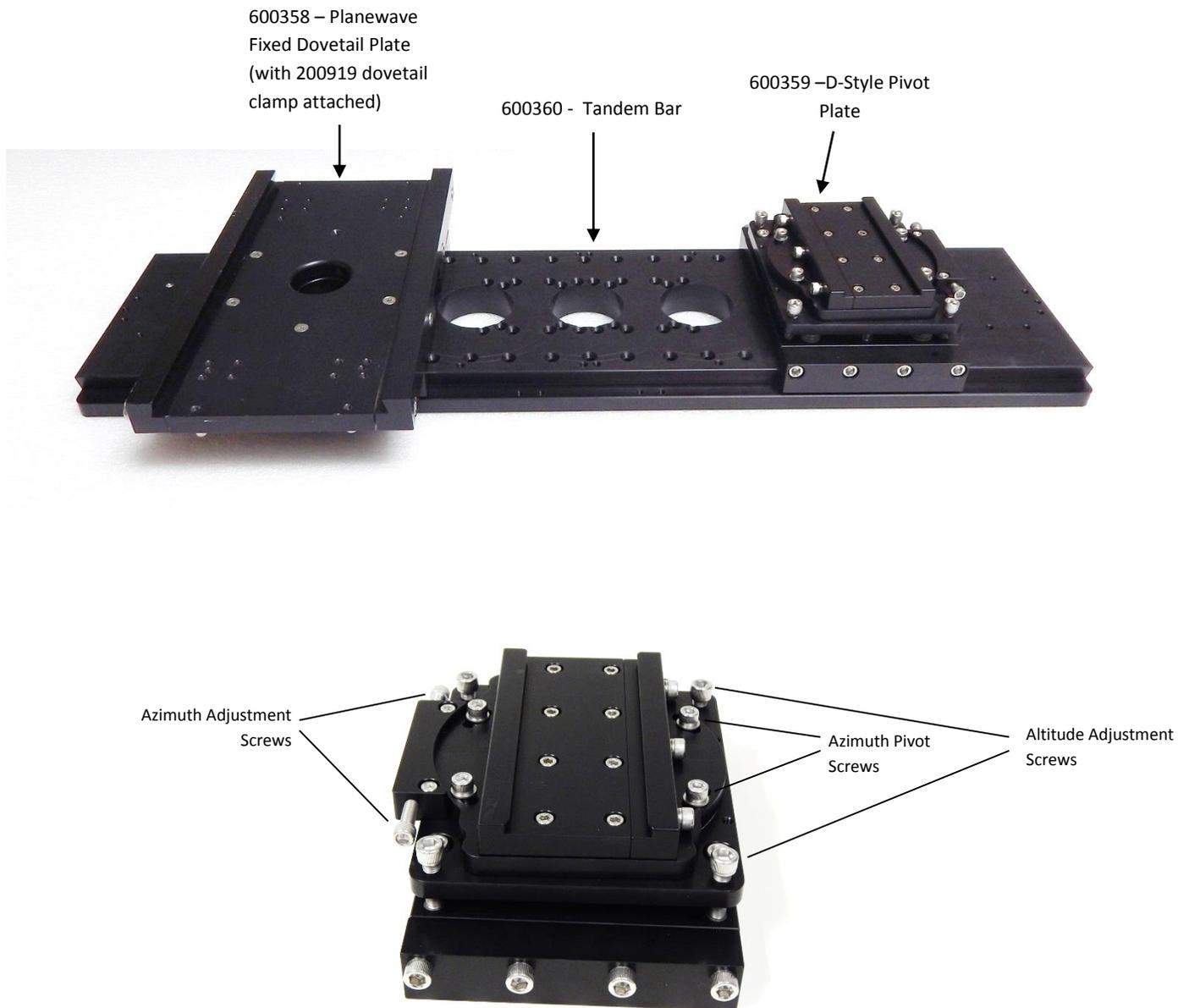
The 600359 –D-Style Pivot Plate mounts directly to the Tandem bar and can hold the CDK12.5 and CDK14 or any telescope using the Losmandy D-Style dovetail mounting bar. The 600359 has both altitude and azimuth adjustment screws which allows you to align the scope to the same position as the main telescope.
