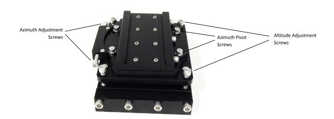
The 600359 –D-Style Pivot Plate mounts directly to the Tandem bar and can hold the CDK12.5 and CDK14 or any telescope using the Losmandy D-Stlye dovetail mounting bar. The 600359 has both altitude and azimuth adjustment screws which allows you to align the scope to the same position as the main telescope.
