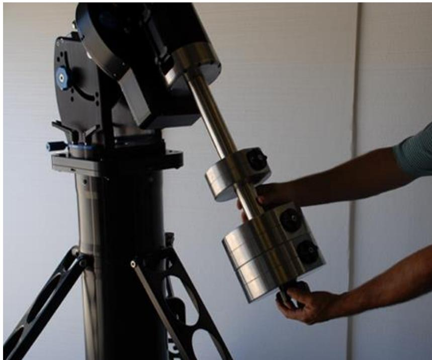
**Figure 12 - Installing the counterweight safety stop**
