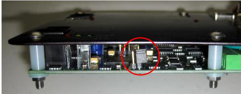
3. Using a pair of needle nose pliers, remove the jumper and re-seat it so that it is bridging both pins.
