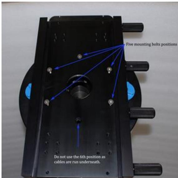
Figure 13 - PlaneWave 7.6" saddle installed
