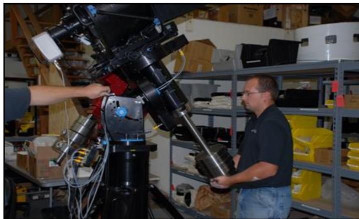
**Figure 9 - If you have to adjust the latitude with a fully loaded mount, you can have one person lift the counterweight bar while you are adjusting the latitude knob. This makes the adjustment much easier.**
