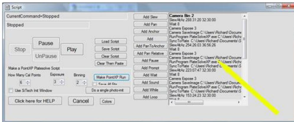
13. Press the PLAY button in the Script window. This will run the script and start the auto mapping run. The PointXP script will cause the telescope to slew to the first calibration point position, take an image, plate solve the image (accurately determine the position of the telescope by comparing the stars in the image to a known star catalog), and add the position information to the mount model.
