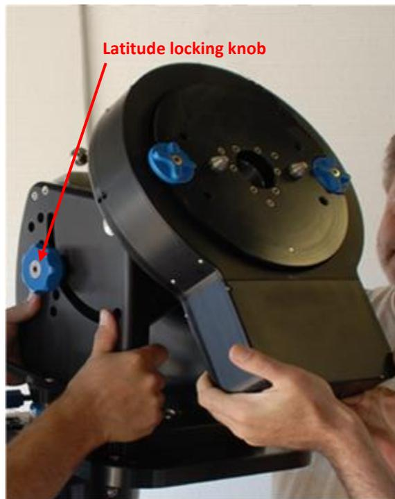
**Figure 5 - Placing the mount base onto the pier**
