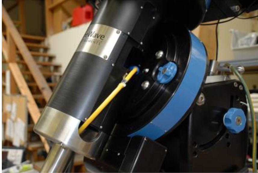
Figure 31 - A cable coming out the bottom of the DEC axis and routed through the top of the RA axis
