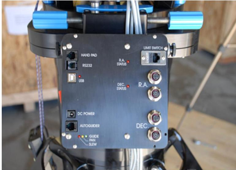
Figure 18 - A200 mount electronics box
