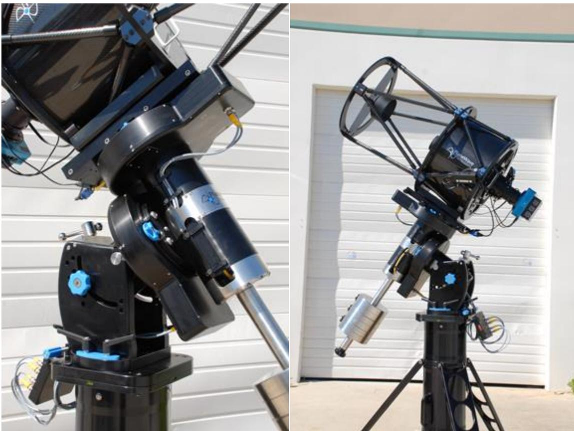
Figure 32 - Cables running through a fully assembled mount
