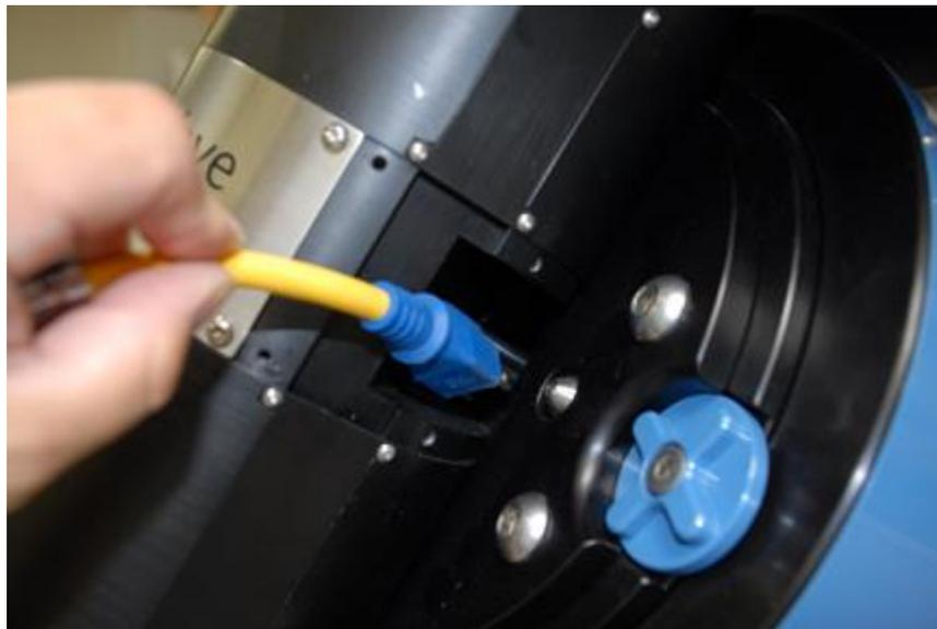
**Figure 29 - Running a cable down from the top of the RA axis**
