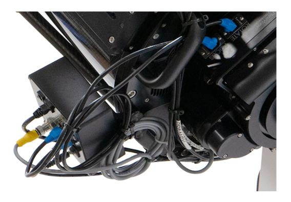
The EFA Electronics box can be attached to several places on the telescope back plate. There are eight ¼-20 threaded holes on the back of the telescope. The EFA mounting bracket, already attached to the electronics box, can be mounted to any one of the eight ¼-20 threaded holes. Use the supplied ¼-20 bolt to attach the EFA box as shown in Picture 2. The mounting position can be varied to accommodate other accessories such as finder scopes to assist with balance.
