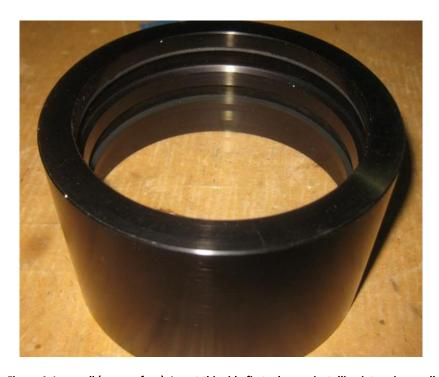
Figure 4: Lens cell (rear surface). Insert this side first when re-installing into mirror cell.
