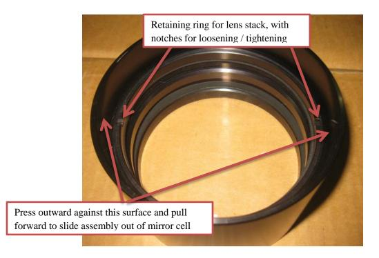
Figure 3: Lens cell (upward facing surface)
