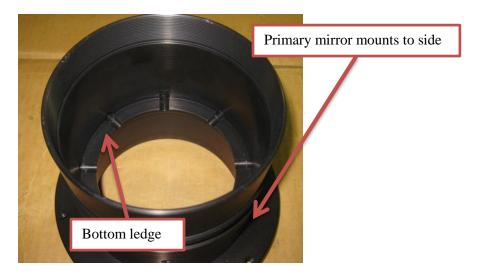
Figure 1: Primary mirror cell with lens group removed
