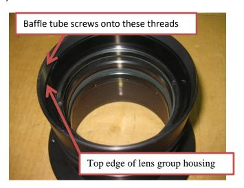
Figure 2: Primary mirror cell with lens group installed
