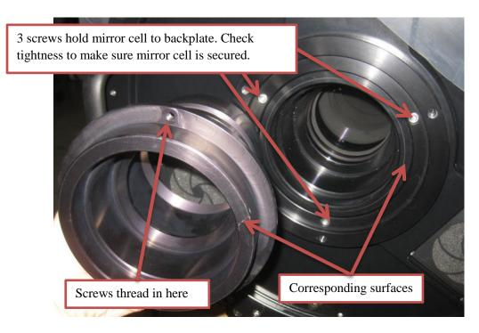
Figure 5: Mirror cell, and corresponding view from back of telescope
