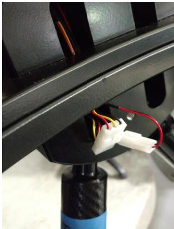
*Figure 16 Temperature sensor and dew heater cables*
