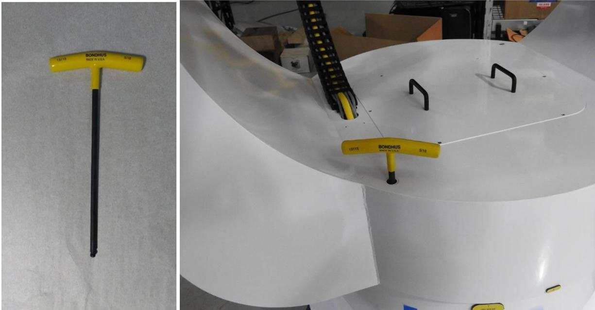
Figure 22 Loosening the azimuth locking ring
