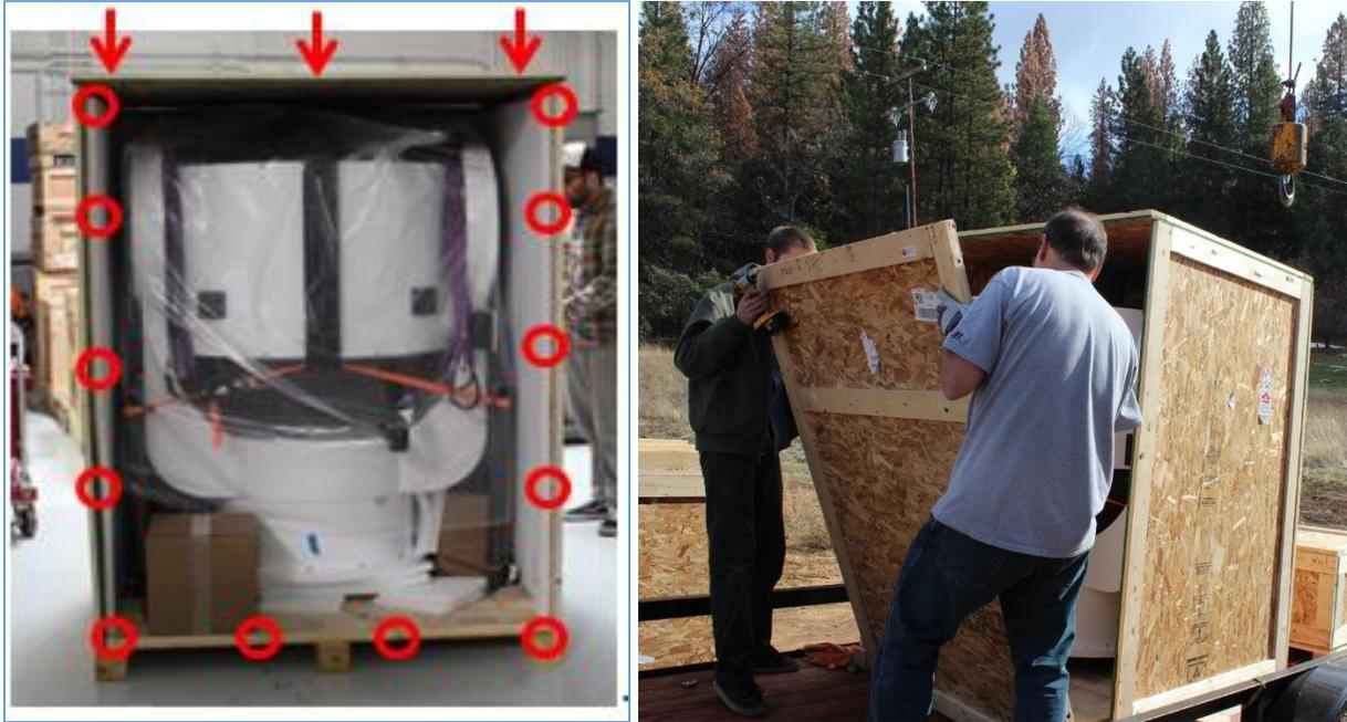
Figure 2 Removing the front panel
