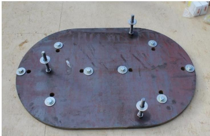
*Figure 9 Pier without cable conduit (the cables will be run along the floor under the telescope)*
