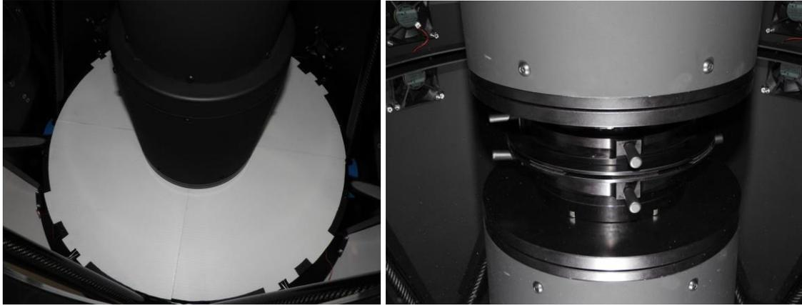
Figure 23 Primary mirror covers and the primary retaining ring
