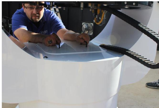
Figure 26 Removing the fork cover
