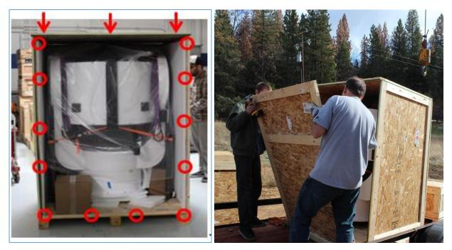
Figure 2 Removing the front panel
