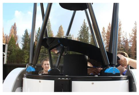
Figure 18 Installing the primary dust cover
