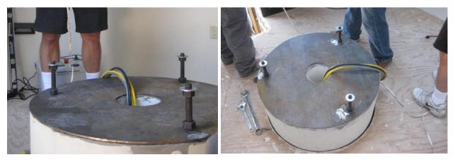
Figure 8 Pier with cable conduit
