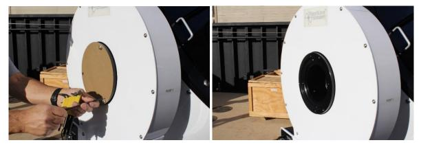
Figure 28 Removing the Nasmyth port covers
