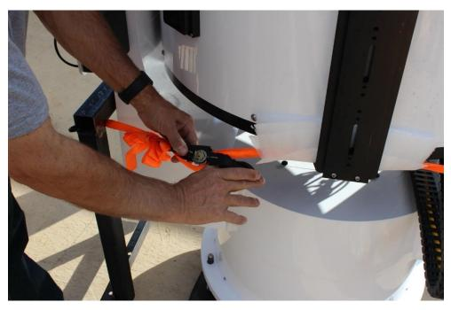
Figure 19 Removing the shipping straps
