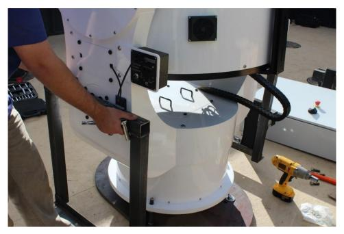
Figure 20 Removing the shipping brackets
