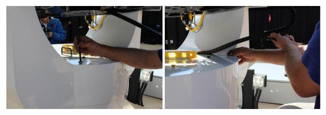
Figure 21 Removing the access hole covers
