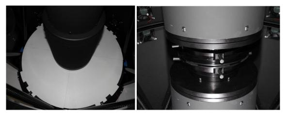
Figure 23 Primary mirror covers and the primary retaining ring
