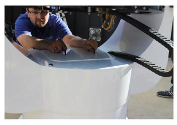
Figure 26 Removing the fork cover
