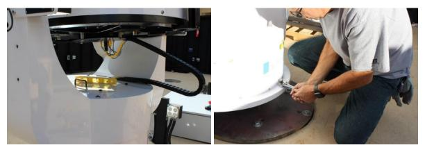
Figure 14 Leveling and securing the base
