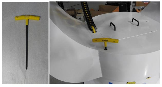
Figure 22 Loosening the azimuth locking ring
