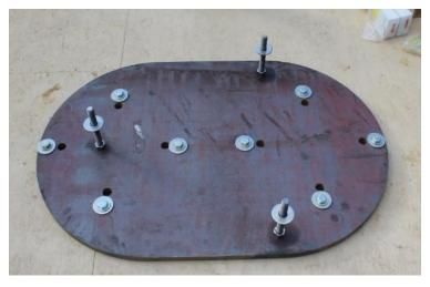
Figure 9 Pier without cable conduit (the cables will be run along the floor under the telescope)
