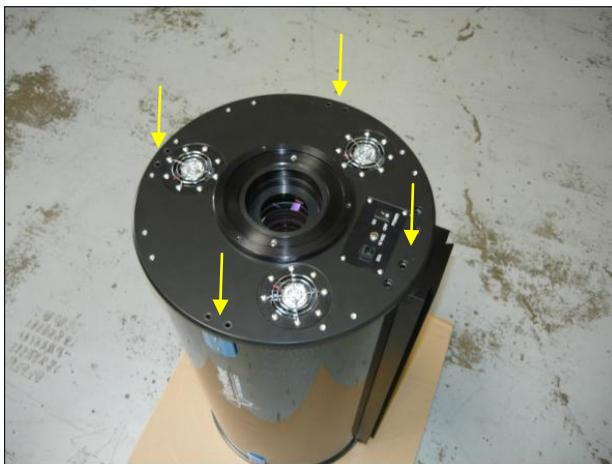
Step 3: Lift up on the side of the back-plate on the opposite side of the dovetail, while holding down the side closest to the dovetail. Then, lift the back-plate up and away from the dovetail (this is so the back of the primary mirror will clear a dovetail mounting block)
