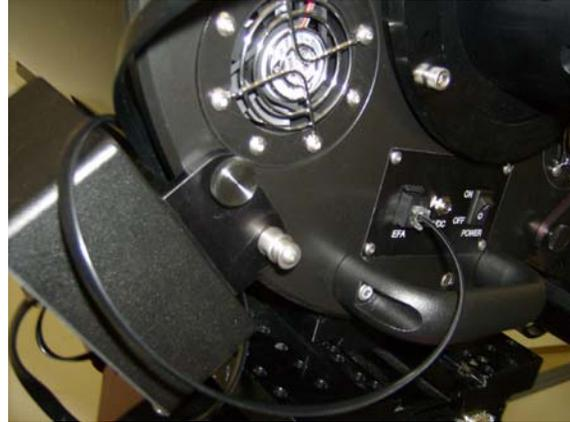
Mount the hand control via the hand control mounting bracket onto the mounting stud.
