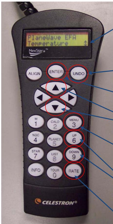
Up/down arrows on the right hand side of the display indicate that there are other menus to scroll to using the scroll up and down buttons (6 and 9)
