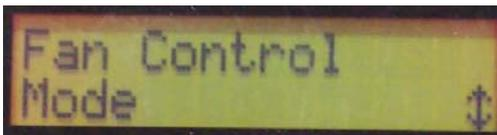
Press the ENTER on the hand control to enter the Mode menu item. There are two items under the fan control mode menu, Relative and Absolute.
