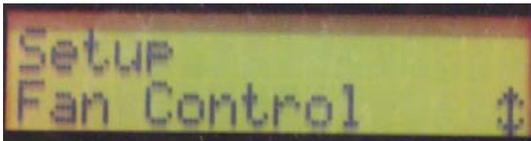
Press the ENTER button on the hand control to enter into the fan control menu.
