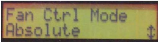
Use this mode if you want the fans to start when the Primary Mirror reaches a set value (see **Temperature** below). Press ENTER on the hand control to select this setting.
