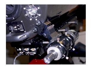
Step 5: Slide the finderscope into the mounting rings. Use the set screws to hold the finder in place. Then slide the female dovetail of the finderscope mounting bracket rings onto the male dovetail mounted on the telescope and use the set screws on the side to set the finderscope mounting bracket rings in place.
