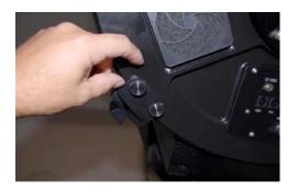
Step 4: Use the two 1/4-20 x 1/2 socket head cap screws with hand knobs attached to mount the mounting bracket to the back plate of the telescope. (on the CDK12.5, if you have the EFA kit, you should not mount the finderscope on the lower left hand set of holes because that is where the EFA kit mounts.
