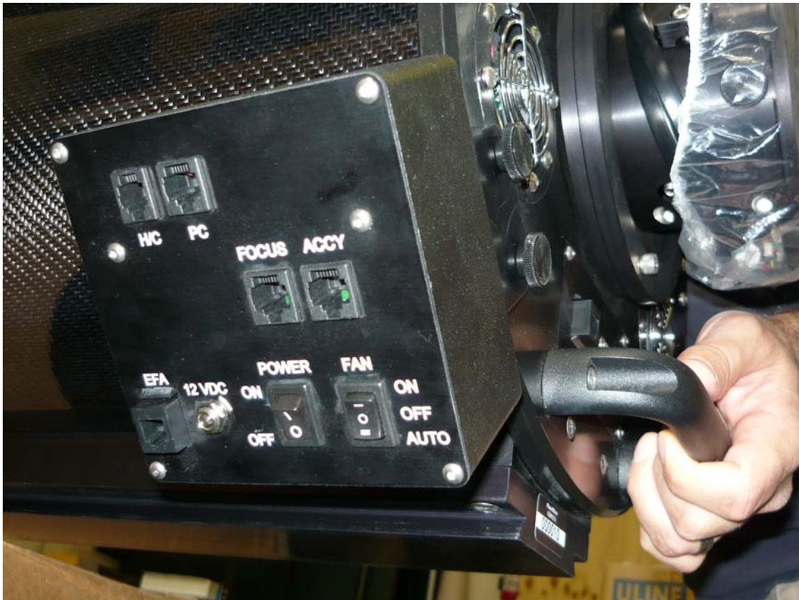
**Picture 2: EFA Box Mounted on the CDK12.5**
