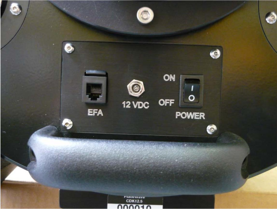
**Picture 3: The CDK12.5 electronics plate**
