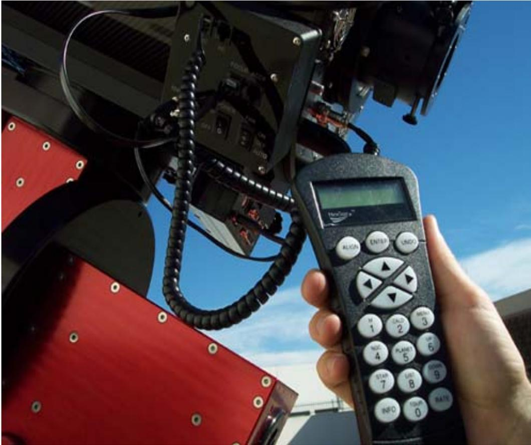
**Picture 4: Hand control plugged into EFA box**
