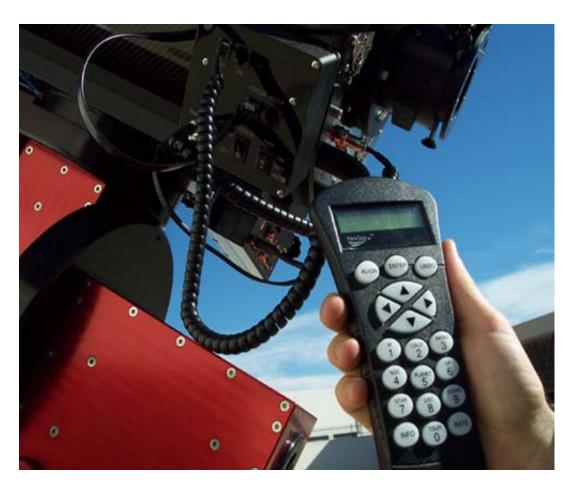
Picture 4: Hand control plugged into EFA box
