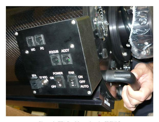
Picture 2: EFA Box Mounted on the CDK12.5
