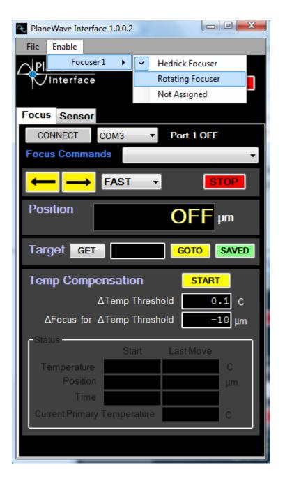
Next connect PWI to the computer. Notice the CONNECT button and the pull down window, in this case showing COM3. It may show multiple COM ports open. Trying selecting one at a time until PWI connects.
