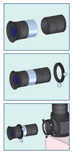
Mount the slit-viewer onto the 20mm guiding eyepiece.
