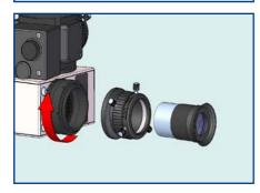
Screw the Baader VariLock extension to the T-2 port of BACHES.
