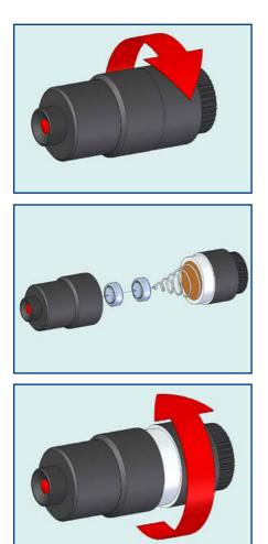
Turn the back of the illuminator counterclockwise approximately three turns to open the battery compartment.
