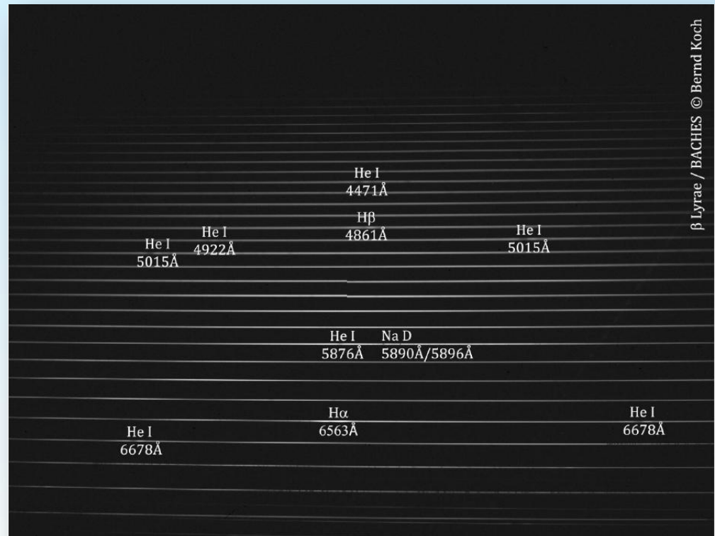
Fig. 2: Spectrum of semi-detached binary system \beta Lyrae, taken on June 8, 2014 at 00:07:24 UT. The spectrum was recorded with BACHES echelle spectrograph and a SBIG ST-8300M CCD camera, Pixel size 10.8 \mu m. This is a single 300s exposure from which a darkframe has been subtracted.
