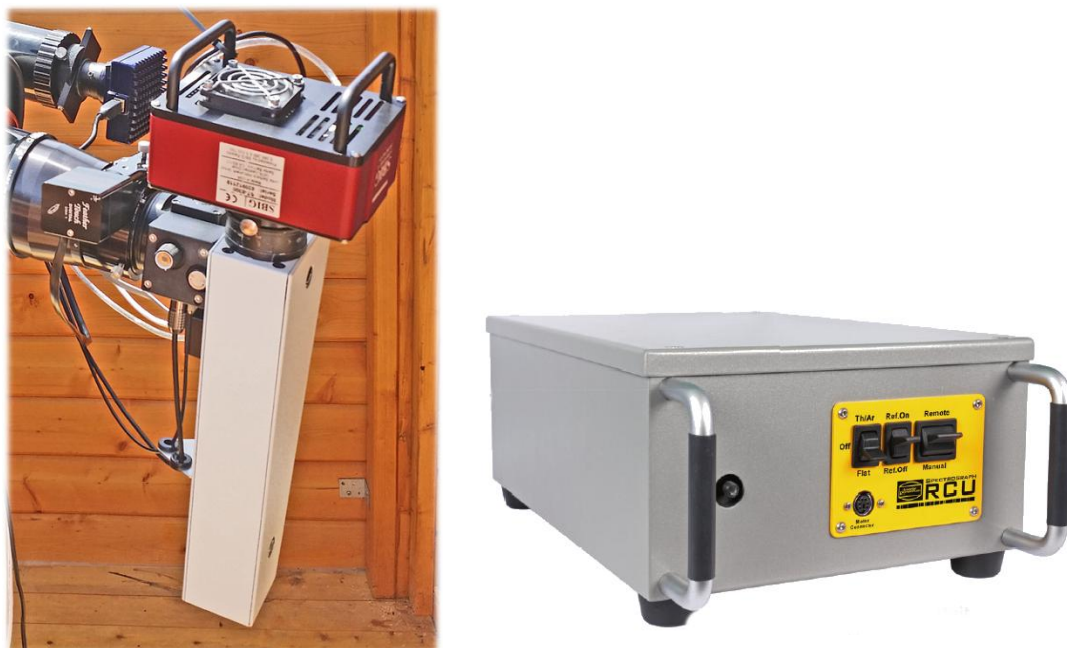
Fig. 1: BACHES echelle spectrograph with attached CCD camera SBIG ST-8300M and fiber connection to Remote Calibration Unit (RCU).
