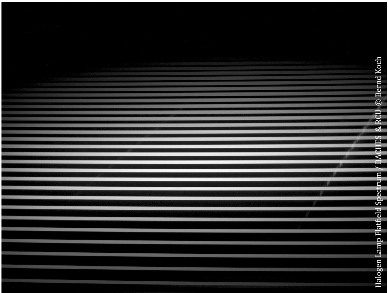
Fig. 4: This halogen lamp flatfield spectrum was supplied by the Remote Calibration Unit (RCU), coupled to the BACHES with a 2.5m glass fiber. The spectrum was taken with the BACHES echelle spectrograph and an SBIG ST-8300M CCD camera, pixel size 10.8 \mu\text{m} . This is a single 20s exposure from which a darkframe has been subtracted.
