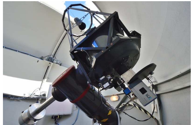
Figure 5. Solaris-4 test-bed setup: ASA mount, OTA and imaging train with photometric camera and spectrograph.
